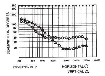
Figure 3: 6-dB-Down Beamwidth versus Frequency
